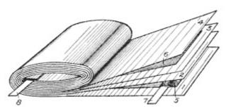
Fig. 121. Rolled Condenser View full size illustration.
