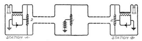
Fig. 136. Current Supply over Parallel Limbs of Line View full size illustration.
