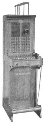
Fig. 294. Upright Magneto Switchboard View full size illustration.
