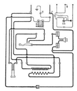
Fig. 175. Circuit of Two-Party Station View full size illustration.
