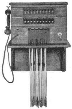
Fig. 303. Sectional Switchboard—Wall Type View full size illustration.
