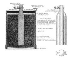
**Fig. 63. Dry Cell** View full size illustration.
