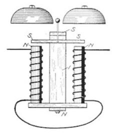
Fig. 21. Polarized Ringer View full size illustration.
