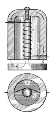
Fig. 94. Iron-Clad Electromagnet View full size illustration.
