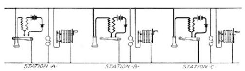
Fig. 168. Metallic Bridging Line View full size illustration.
