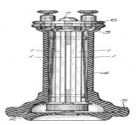
Fig. 49. Single-Pole Receiver View full size illustration.
