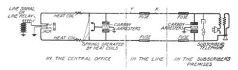
Fig. 225. Complete Line Protection
