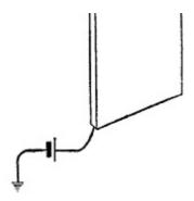
Fig. 119. Condenser Plate View full size illustration.
