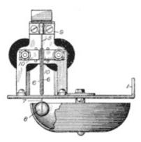
Fig. 178. Under-Tuned Ringer View full size illustration.
