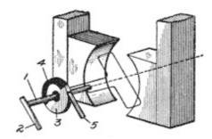
Fig. 77. Pulsating-Current Commutator View full size illustration.
