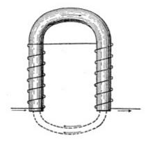
**Fig. 92. Horseshoe Electromagnet** View full size illustration.
