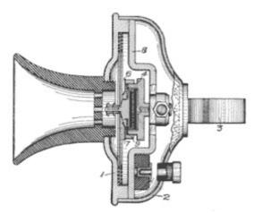
Fig. 40. White Solid-Back Transmitter View full size illustration.
