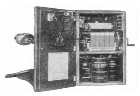
Fig. 143. Magneto Wall Set View full size illustration.
