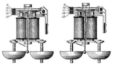
**Fig. 199. Broken-Back Ringer** View full size illustration.
