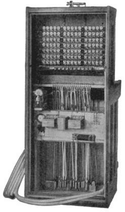
Fig. 300. Rear View of Target Signal, Magneto Switchboard View full size illustration.
