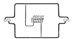
Fig. 281. Bridging Drop-Cord Circuit View full size illustration.
