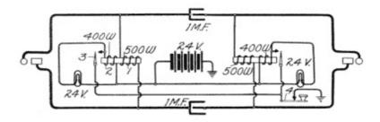
Fig. 291. Cord Circuit with Double Lamp Signals
