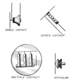
Fig. 9. General Types of Transmitters View full size illustration.
