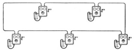
Fig. 164. Metallic-Circuit Series Line View full size illustration.
