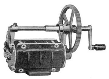
Fig. 72. Generator with Magnets Removed View full size illustration.
