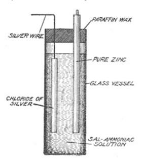
Fig. 66. Chloride of Silver Cell View full size illustration.
