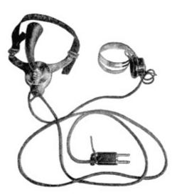
Fig. 272. Operator's Talking Set View full size illustration.
