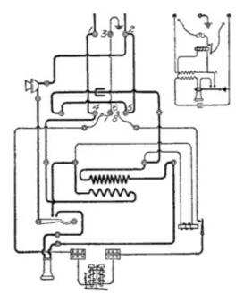
Fig. 177. Circuit of Four-Party Station with Relay View full size illustration.
