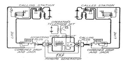
Fig. 273. Circuit of Simple Magneto Switchboard View full size illustration.
