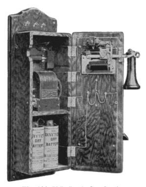
Fig. 190. K.B. Lock-Out Station
