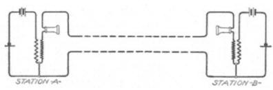
Fig. 127. Local-Battery Stations with Metallic Circuit View full size illustration.
