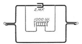
Fig. 282. Series Drop-Cord Circuit View full size illustration.
