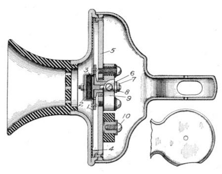
Fig. 43. Kellogg Transmitter View full size illustration.
