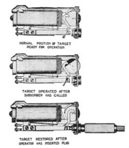
Fig. 254. Western Electric Drop and Jack View full size illustration.
