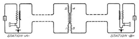
Fig. 130. Bridging Battery with Repeating Coil View full size illustration.
