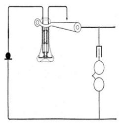
Fig. 162. Monarch Common-Battery Wall Set View full size illustration.
