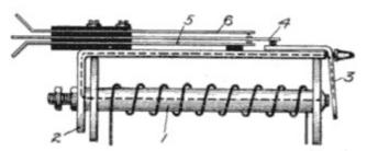
Fig. 95. Electromagnet of Relay View full size illustration.
