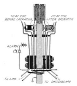
Fig. 227. Self-Soldering Heat-Coil Arrester View full size illustration.
