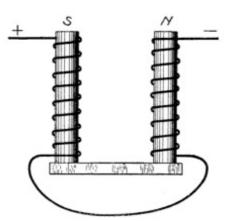
**Fig. 20. Electromagnet** View full size illustration.
