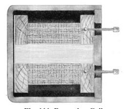
Fig. 111. Repeating Coil View full size illustration.
