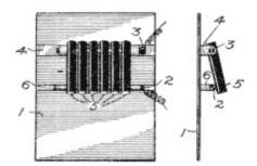
Fig. 39. Multiple-Electrode Transmitter View full size illustration.
