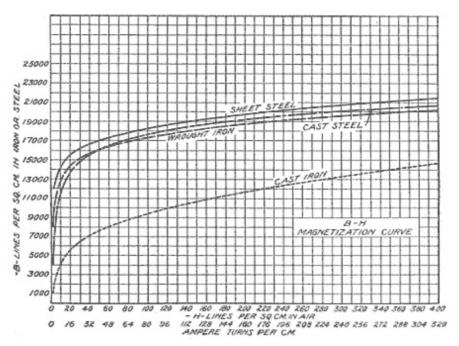
Fig. 89. Magnetization Curve View full size illustration.
