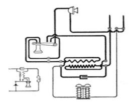
Fig. 153. Stromberg-Carlson Common-Battery Wall Set View full size illustration.
