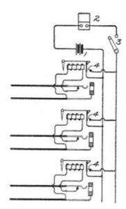
Fig. 274. Night-Alarm Circuit View full size illustration.
