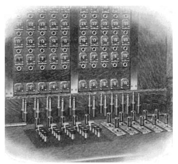
Fig. 296. Details of Drop, Jack, Plug, and Key Arrangement View full size illustration.
