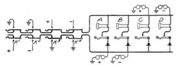
Fig. 172. Four-Party Polarity Selection View full size illustration.
