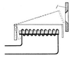
Fig. 23. Electromagnetic Visible Signal View full size illustration.
