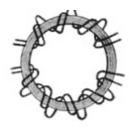
**Fig. 112. Diagram of Toroidal Repeating Coil** View full size illustration.
