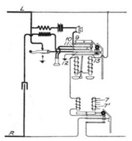
Fig. 200. Details of Ringer Connection View full size illustration.
