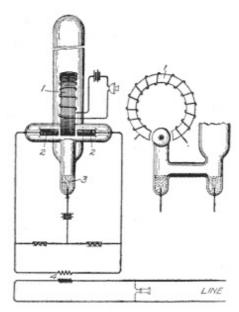
Fig. 37. Mercury-Arc Telephone Relay View full size illustration.
