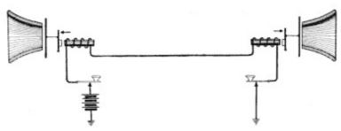
Fig. 6. Telegraph Equipment Converted into Telephone Equipment View full size illustration.
