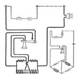
**Circuits of Common-Battery Telephone Sets.** The complete circuits of the Kellogg desk-stand arrangement are shown in Fig. 160, the desk-stand parts being shown at the left and the bell-box parts at the right. As is seen, but two conductors extend from the former to the latter. A simplified theoretical sketch is also shown in the upper right-hand corner of this figure.
