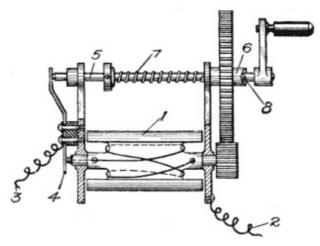
**Fig. 74. Generator Shunt Switch** View full size illustration.
