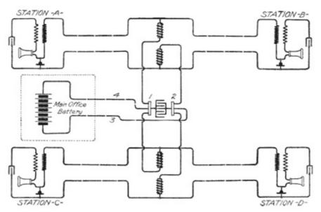
Fig. 141. Current Supply from Distant Point View full size illustration.
