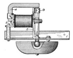
Fig. 179. Under-Tuned Ringer View full size illustration.
