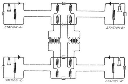
Fig. 140. Two Sources for Many Lines View full size illustration.
