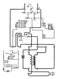
Fig. 176. Circuit of Four-Party Station without Relay View full size illustration.
