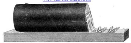
Fig. 110. Repeating Coil View full size illustration.
