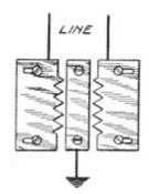
Fig. 203. Saw Tooth Arrester View full size illustration.
