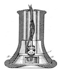
Fig. 52. Automatic Electric Company Direct-Current Receiver View full size illustration.
