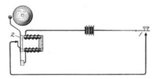
Fig. 16. Vibrating Bell View full size illustration.
