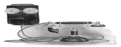
Fig. 159. Microtelephone Set View full size illustration.
