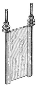
Fig. 117. Mica Card Resistance View full size illustration.
