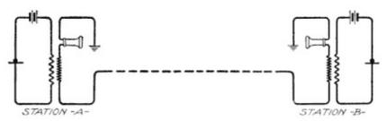
Fig. 125. Local-Battery Stations with Grounded Circuit View full size illustration.
