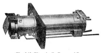
Fig. 263. Electrically Restored Drop
