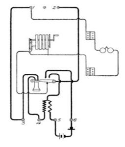
Fig. 147. Circuit of Series Magneto Set View full size illustration.
