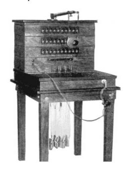
Fig. 305. Sectional Switchboard—Table Type View full size illustration.
