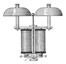
Fig. 80. Polarized Bell View full size illustration.
