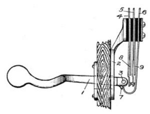
**Fig. 84. Short Lever Hook Switch** View full size illustration.
