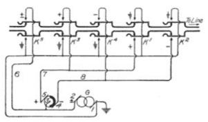
Fig. 174. Ringing-Key Arrangement View full size illustration.
