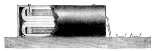
Fig. 109. Repeating Coil View full size illustration.
