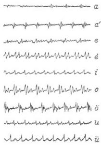
Fig. 14. Oscillogram of Telephone Currents
