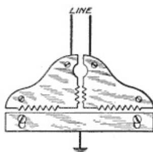
**Fig. 204. Saw-Tooth Arrester**
