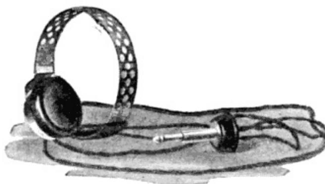
**Fig. 58. Operator's Receiver and Cord**
