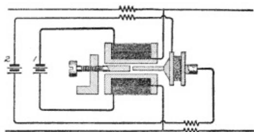
**Fig. 36. Shreeve Repeater and Circuit**
