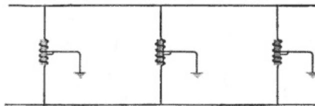
**Fig. 232. Drainage Coils**
