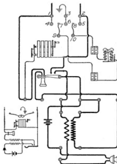
**Fig. 176. Circuit of Four-Party Station without Relay**
