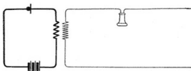
**Fig. 12. Conventional Diagram of Talking Circuit**
