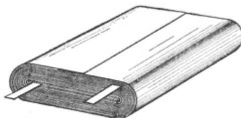
**Fig. 122. Rolled Condenser**
