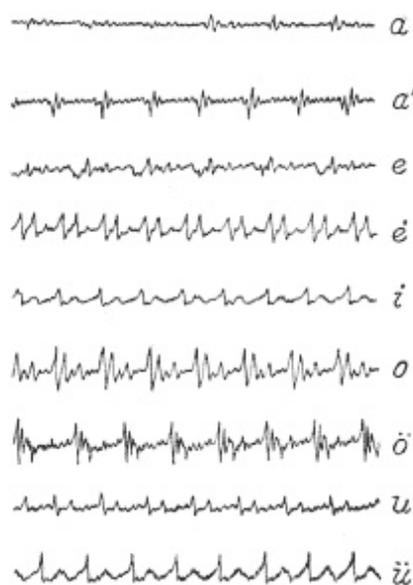
**Fig. 14. Oscillogram of Telephone Currents**
