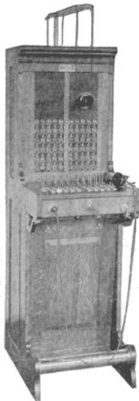
**Fig. 294. Upright Magneto Switchboard**
