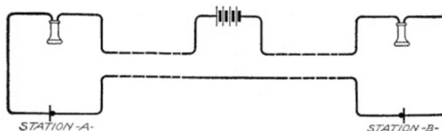
**Fig. 129. Battery in Series with Two Lines**
