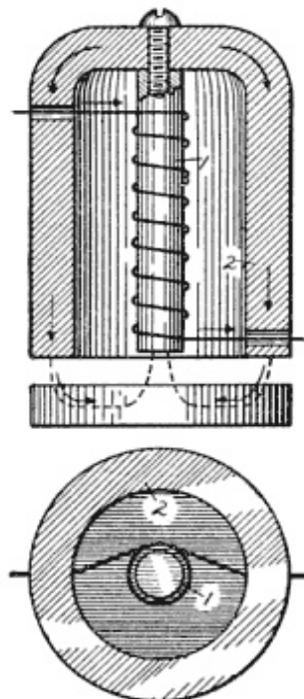
**Fig. 94. Iron-Clad Electromagnet**[View full size illustration.](#)
