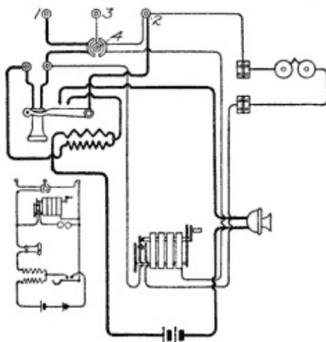
**Fig. 149. Circuit of Bridging Magneto Set**
