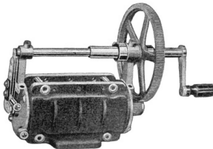
**Fig. 72. Generator with Magnets Removed**
