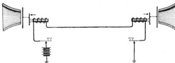
**Fig. 6. Telegraph Equipment Converted into Telephone Equipment**
