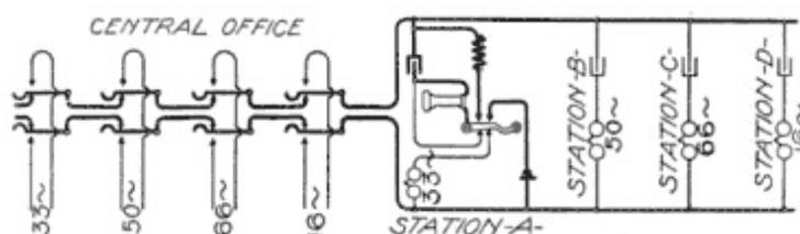
Fig. 185. Circuits of Kellogg Harmonic System
