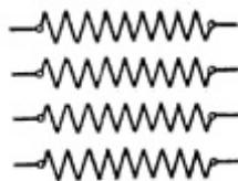
**Fig. 116. Symbol of Four-Winding Repeating Coil**
