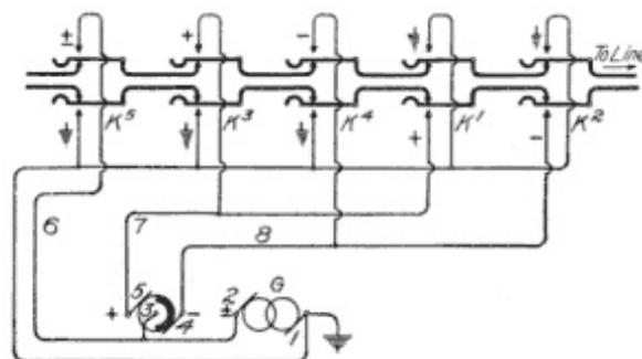
**Fig. 174. Ringing-Key Arrangement**
