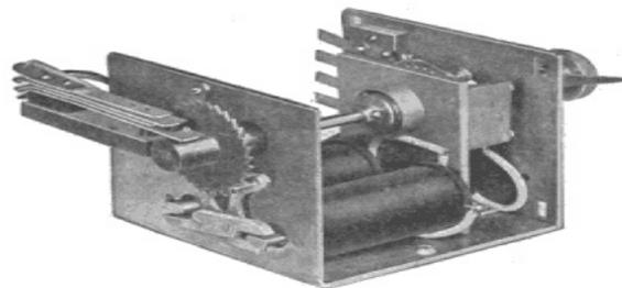
**Fig. 201. Central-Office Impulse Transmitter**
