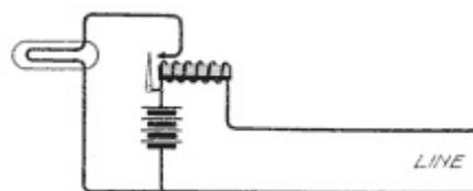
**Fig. 25. Lamp Signal Controlled by Relay**
