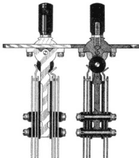
**Fig. 267. Vertical-Spring Listening and Ringing Key**
