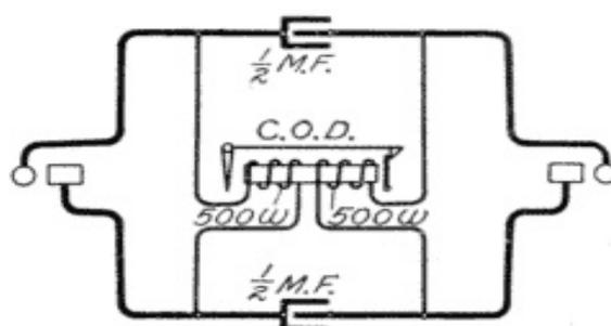
**Fig. 285. Non-Ring-Through Cord Circuit**[View full size illustration.](#)
