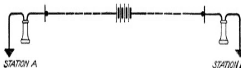
**Fig. 128. Battery in Series with Two Lines**
