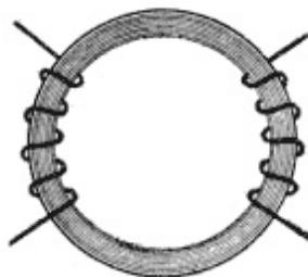
**Fig. 104. Symbol of Toroidal Impedance Coil**
