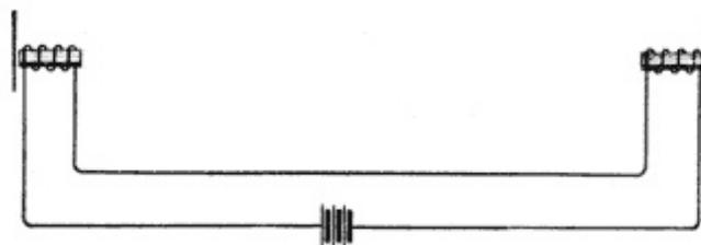
**Fig. 3. Magneto Telephones without Permanent Magnets**
