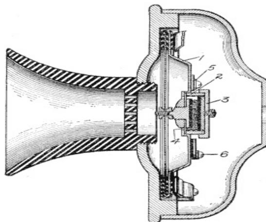
**Fig. 42. New Western Electric Transmitter**
