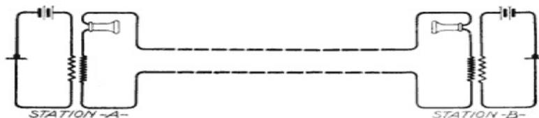
**Fig. 126. Local-Battery Stations with Metallic Circuit**
