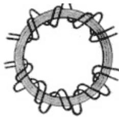
**Fig. 112. Diagram of Toroidal Repeating Coil**
