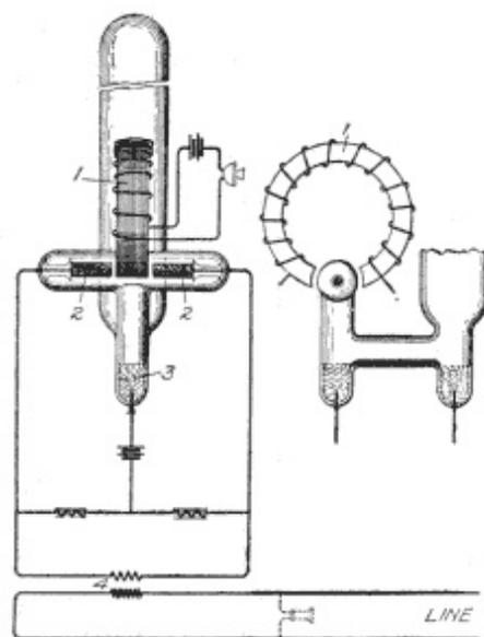
**Fig. 37. Mercury-Arc Telephone Relay**
