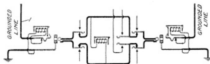
**Fig. 277. Connection Between Grounded Lines**
