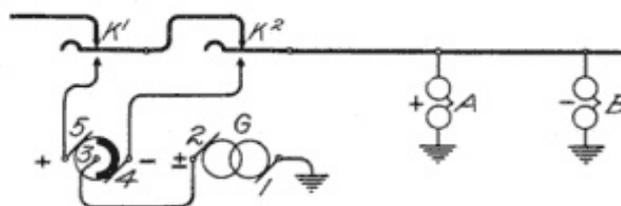
Fig. 171. Principle of Selection by Polarity
