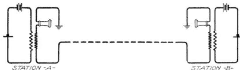
Fig. 125. Local-Battery Stations with Grounded Circuit
