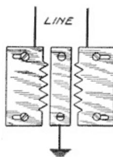
**Fig. 203. Saw Tooth Arrester**
