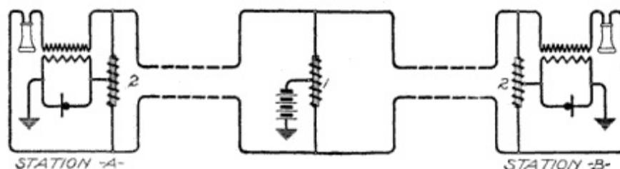
**Fig. 136. Current Supply over Parallel Limbs of Line**
