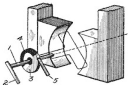
**Fig. 77. Pulsating-Current Commutator**
