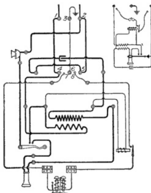
**Fig. 177. Circuit of Four-Party Station with Relay**
