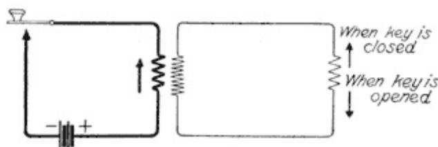
**Fig. 13. Induction-Coil Action**
