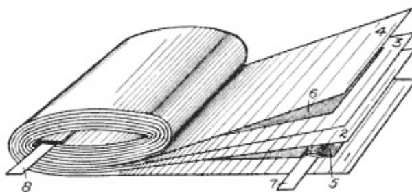
**Fig. 121. Rolled Condenser**
