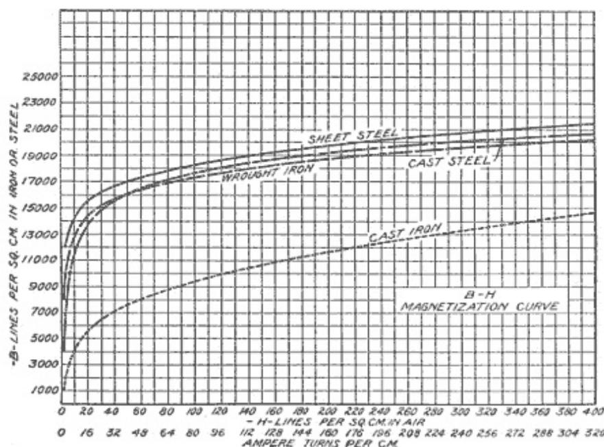
**Fig. 89. Magnetization Curve**
