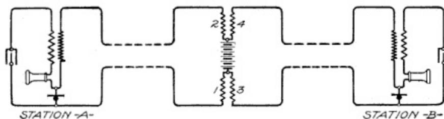
**Fig. 130. Bridging Battery with Repeating Coil**
