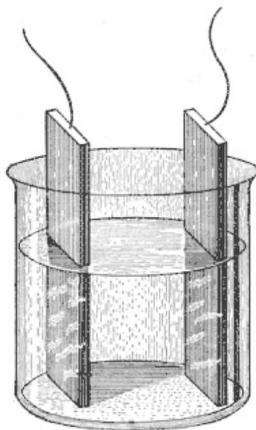
**Fig. 60. Simple Voltaic Cell**[View full size illustration.](#)
