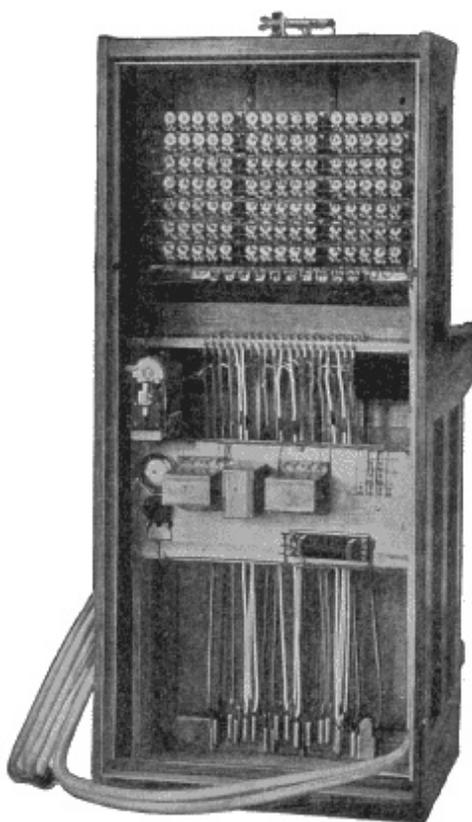
**Fig. 300. Rear View of Target Signal, Magneto Switchboard**
