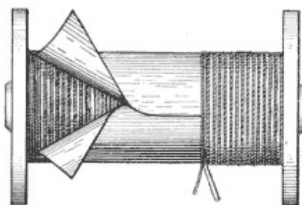
**Fig. 99. Electromagnet with Bare Wire**
