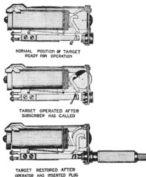
**Fig. 254. Western Electric Drop and Jack**[View full size illustration.](#)
