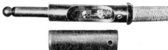
**Fig. 264. Switchboard Plug**
