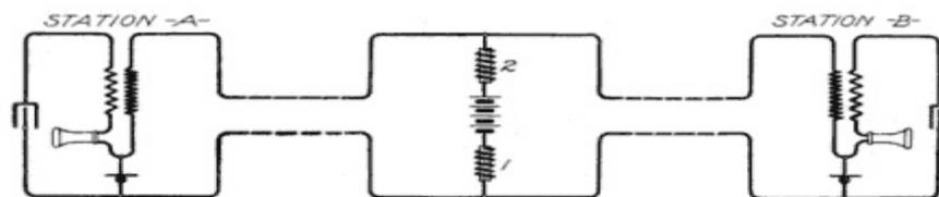
**Fig. 131. Bridging Battery with Impedance Coils**
