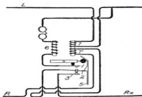
**Fig. 198. Details of Latching Relay Connections**
