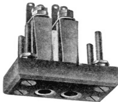
**Fig. 271. Operator's Cut-in Jack**
