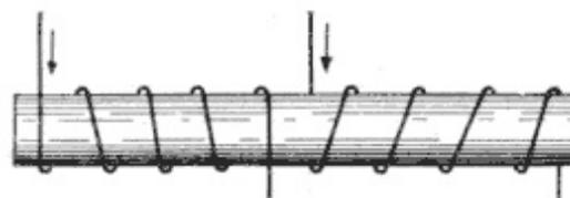
**Fig. 97. Tandem Differential Electromagnet**
