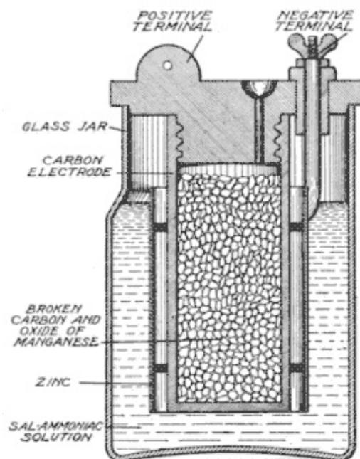
**Fig. 62. Carbon Cylinder LeClanché Cell**
