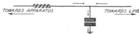
**Fig. 213. Impedance and Air-Gap**
