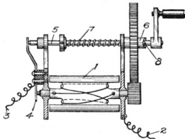
**Fig. 74. Generator Shunt Switch**
