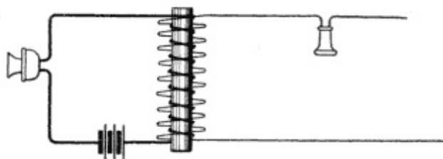
**Fig. 11. Battery in Local Circuit**
