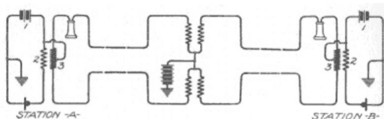
**Fig. 137. Current Supply over Parallel Limbs of Line**
