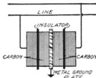
**Fig. 205. Carbon Block Arrester**
