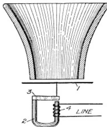
**Fig. 1. Type of Magneto Telephone**
