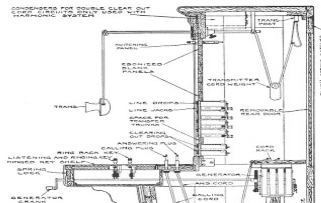
**Fig. 297. Cross-Section of Upright Switchboard (partial)**
