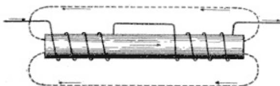
**Fig. 91. Bar Electromagnet**
