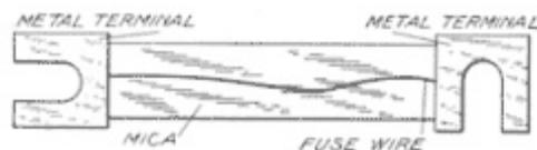
**Fig. 216. Mica Slip Fuse**
