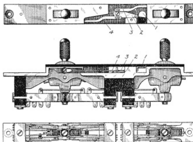
**Fig. 266. Horizontal-Spring Listening and Ringing Key**
