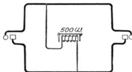
**Fig. 281. Bridging Drop-Cord Circuit**
