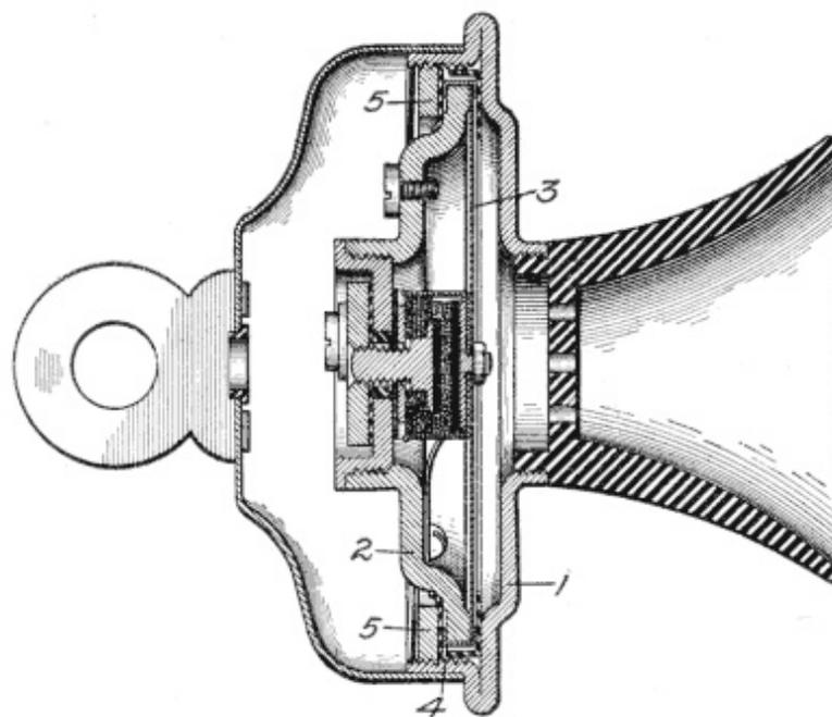
**Fig. 44. Automatic Electric Company Transmitter**
