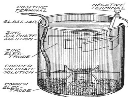
**Fig. 64. Gravity Cell**
