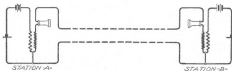
**Fig. 127. Local-Battery Stations with Metallic Circuit**
