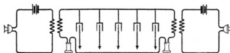
**Fig. 31. Test of Line with Varying Shunt Capacity**
