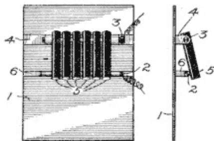
**Fig. 39. Multiple-Electrode Transmitter**
