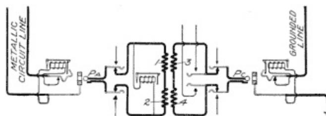
**Fig. 279. Connection of Dissimilar Lines through Repeating Coil**
