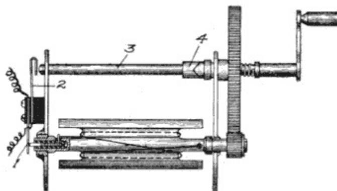
**Fig. 75. Generator Cut-in Switch**
