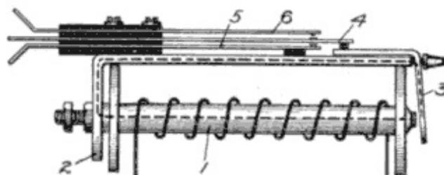
**Fig. 95. Electromagnet of Relay**[View full size illustration.](#)
