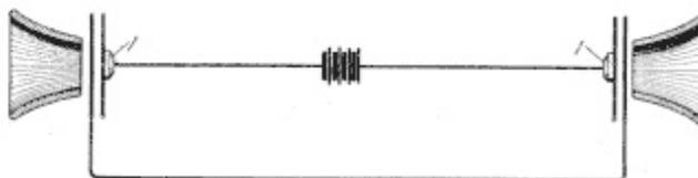
**Fig. 7. Electrostatic Telephone**
