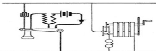
**Fig. 169. Circuits of Bridging Station**
