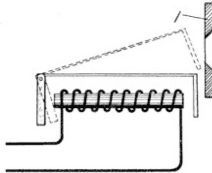
**Fig. 23. Electromagnetic Visible Signal**
