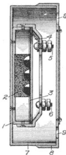
**Fig. 46. Acousticon Transmitter**
