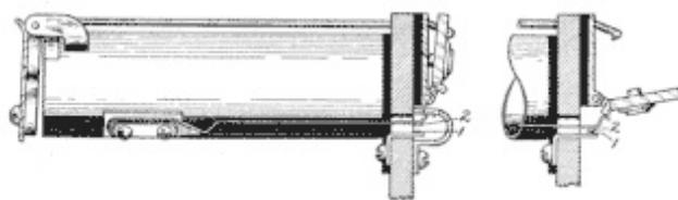
**Fig. 249. Drop with Night-Alarm Contacts**
