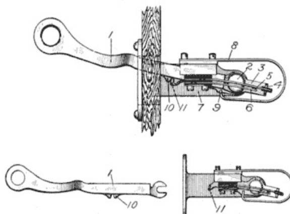
**Fig. 85. Removable Lever Hook Switch**
