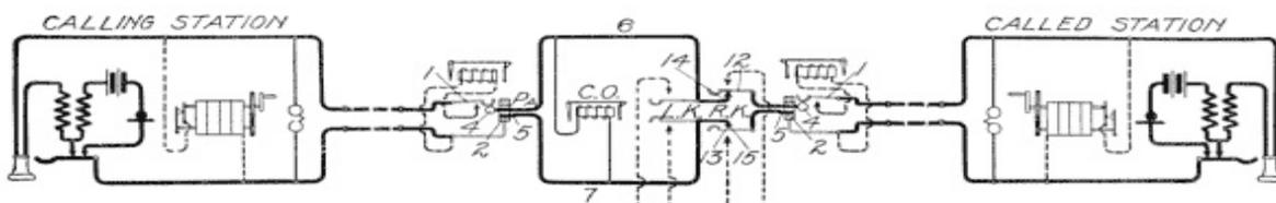
**Fig. 244. Subscribers Connected for Conversation**
