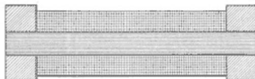
**Fig. 101. Section of Open-Circuit Impedance Coil**
